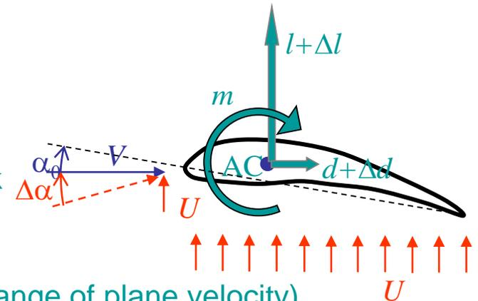
$$\Delta L \simeq \frac{\rho V^2 S \partial_\alpha C_{L\text{plane}} \Delta\alpha}{2} \simeq \frac{\rho V S C_{L\alpha\text{plane}} U}{2}$$
