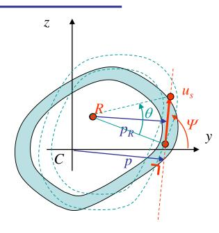
Twist & Warping under pure torsion
