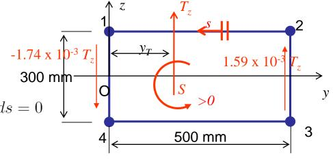
$$\begin{array}{l} \bullet \quad \text{With} \quad \oint \frac{q_0\left(s\right)}{t} \; ds = q_0^{14} \times \frac{l^{14}}{t_{14}} + q_0^{32} \times \frac{l^{32}}{t_{32}} \\ \\ = -1.74 \times 10^{-3} \, T_z \times \frac{300}{10} + 1.59 \times 10^{-3} \, T_z \times \frac{300}{8} = 7.425 \times 10^{-3} \, T_z \\ \\ \text{and} \quad \oint \frac{1}{t} \; ds = 2 \times \frac{500}{10} + \frac{300}{10} + \frac{300}{8} = 167.5 \end{array}$$
