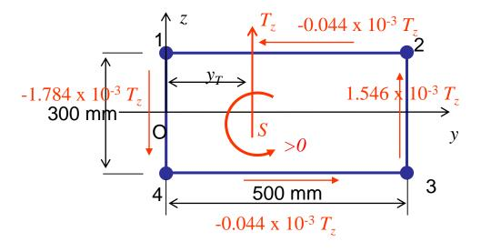
$$y_T T_z = 1.546 \times 10^{-3} T_z \times 300 \times 500 - 2 \times 0.044 \times 10^{-3} T_z \times 500 \times 150$$
