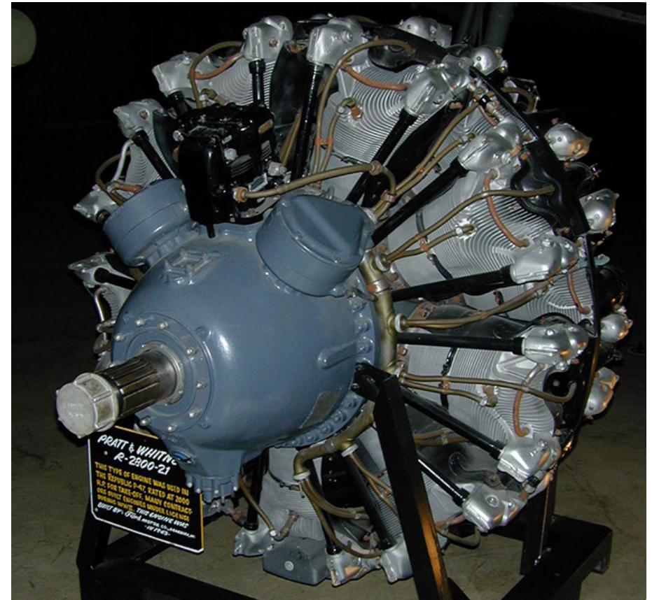
Pratt & Whitney R-2800 Double Wasp. Air-cooled, twin-row radial engine with 18 cylinders. Power: 1500 hp (1939) to 2800 (with turbocharger, 1945)
