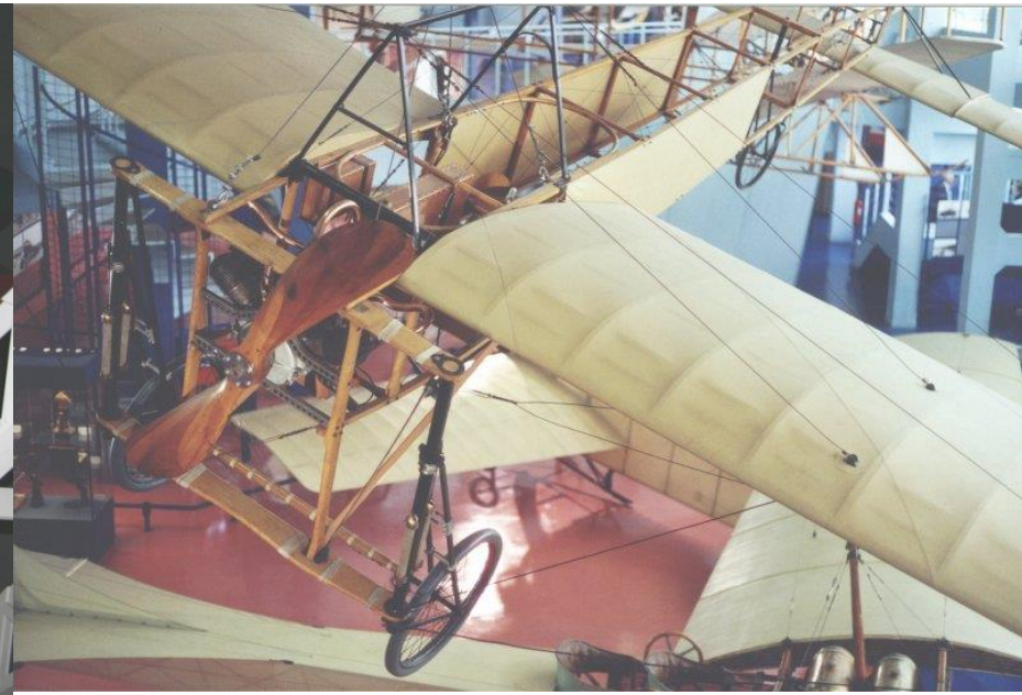
Figure 1-5 Wood-and-fabric-type wing structure
