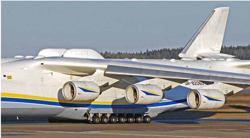
Antonov 225: fuselage fairings
