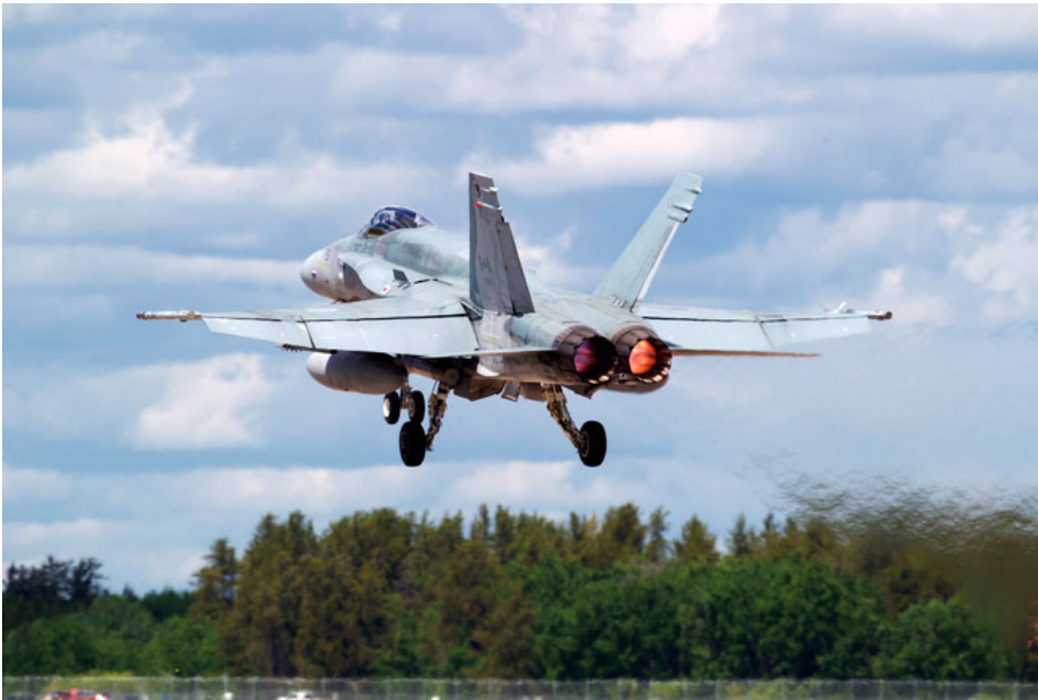
Rudder toe-in during take-off for the F-18
