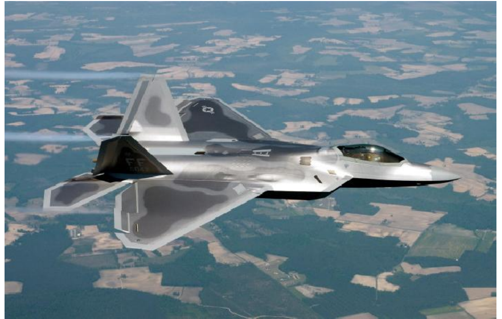
Rudder toe-out in-flight for braking for the F-22
